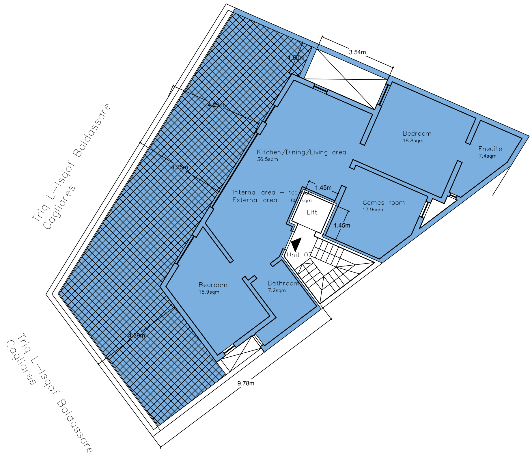
Proposed Receded Floor Level Plan Scale 1:100 clean copy
